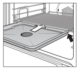
The grill pan is ideal for catching drippings from meat or poultry roasted or grilled directly on the rack. Slide the roasting pan onto the rail below the wire rack. See illustration.
